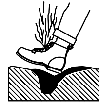
4. FINISH FILLING IN SOIL. FIRM WITH HEEL.
