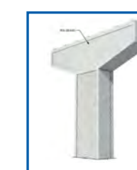
Bridge Pier Hammer Head With Rectangular Column
